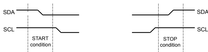
Figure 16-3. START and STOP Conditions
